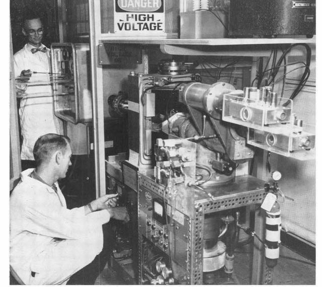
G. W. McCLURE (5152), standing, indicates where 5152). Magnet analyzes and splits beam into different types of ions, and then directs the ions are produced in microbevatron before passing desired type into the experimental apparatus. through magnet beside Dwight Allensworth (also
